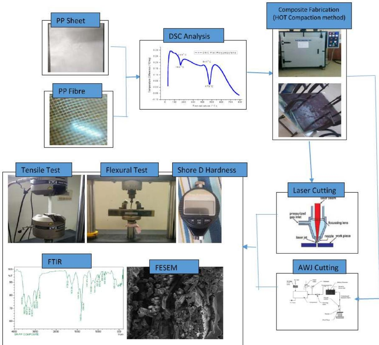
Figure 2: Schematic diagram of fabrication and testing
