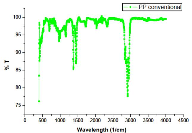
Figure 7: FTIR Plot of PP Conventional cut sample
