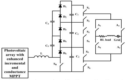
Fig. 1 Proposed grid connected system using multilevel inverter with multi output boost converter
