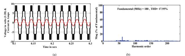
Fig. 6. (a) Output voltage and current waveform with filter (b) Harmonic spectrum plot for output voltage
