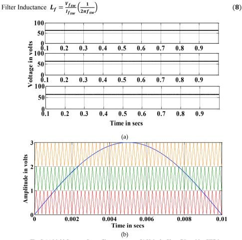
Fig. 5. (a) Multi Output voltage of boost converter (b) Unipolar Phase Disposition PWM
