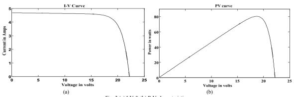
Fig. 3 (a) I-V & (b) P-V characteristics
