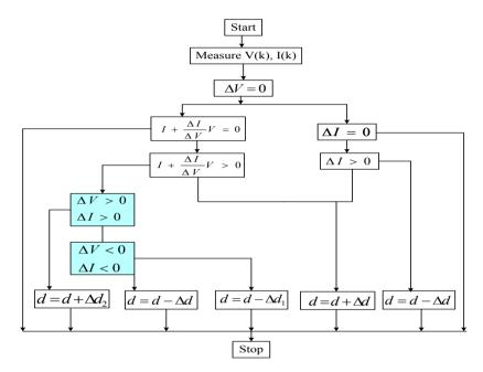
Fig. 4 Improved Incremental and Conductance MPPT algorithm
