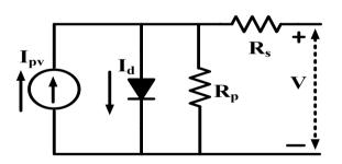
Fig. 2 Single diode model equivalent circuit
