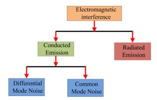
**FIGURE 3.** Classification of electromagnetic interference in an electrical circuit.
