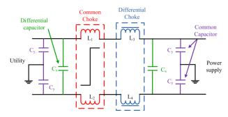
FIGURE 4. Schematic circuit diagram of passive EMI filter.
