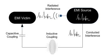
**FIGURE 2.** Schematic block diagram of electromagnetic interference (EMI) coupling path.
