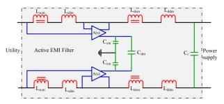
FIGURE 5. Schematic circuit diagram of active EMI filter.
