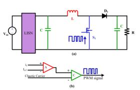
**FIGURE 10.** (a) Schematic circuit diagram of chaotic PWM boost converter, (b) block diagram for chaotic PWM pulse generation.
