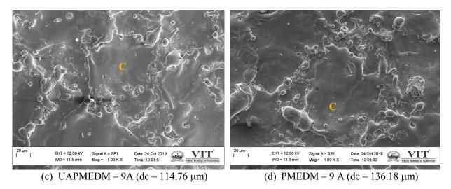
Figure 6. Influence of peak current and ultrasonic vibration on crater diameter (C - crater).
