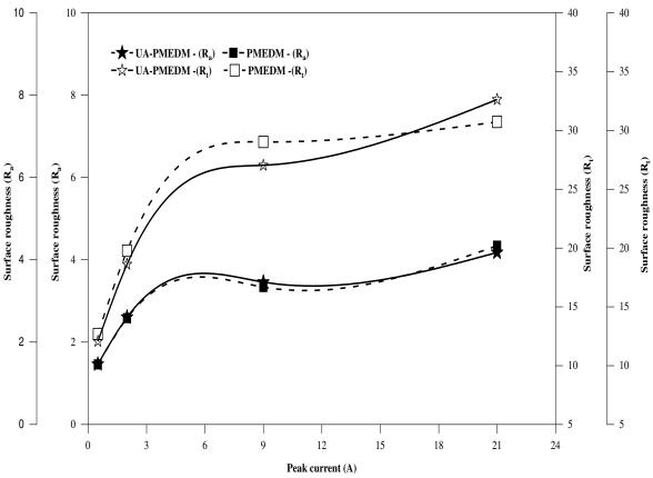
Figure 3. Influence of peak current on surface roughness.
