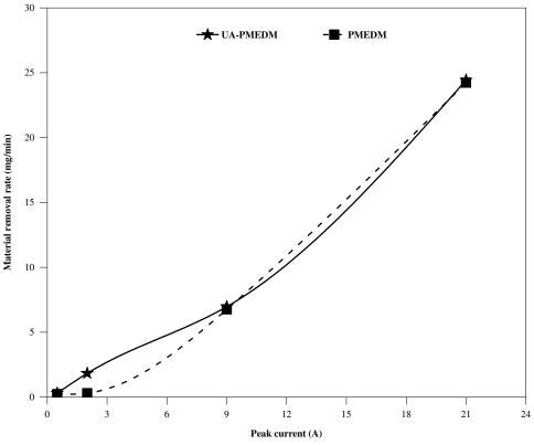
Figure 2. Influence of Peak current on material removal rate.
