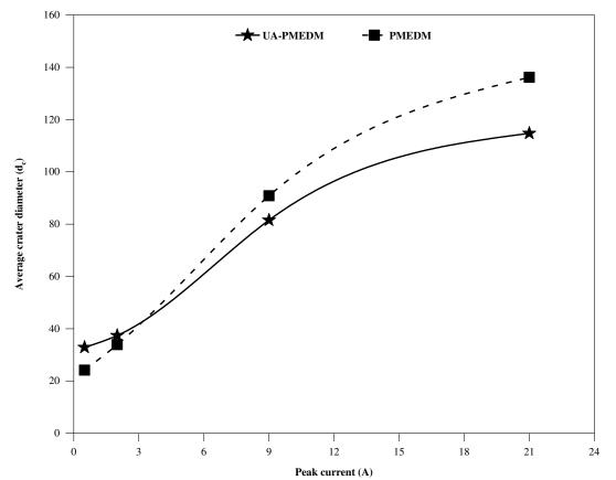
Figure 5. Peak current Vs Average crater diameter (d<sub>c</sub>).
