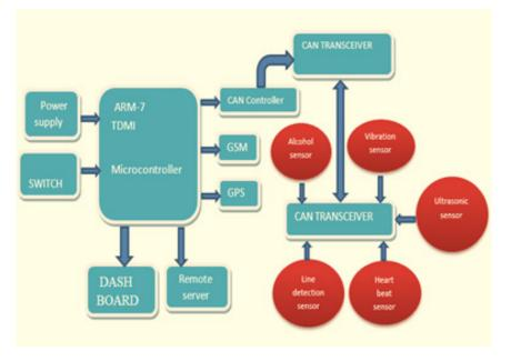
Figure 4. Block diagram.
