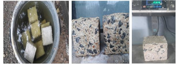
Figure 1. Specimens in acid solution and its testing
