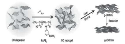
**Figure 6.** Preparation of graphene oxide film. Reproduced with permission from [64]. Copyright 2014 John Wiley and Sons.
