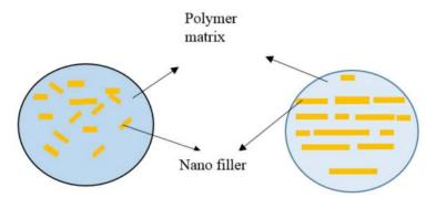
Figure 7. Conventional and bio-inspired nano composite structure.
