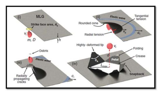
**Figure 1.** Penetration process (i) initial stage; (ii) cone formation stage; (iii) fracture stage; and (iv) post penetration stage, MLG: Multilayer graphene,  $V_i$  (impact speed),  $V_c$  (radial speed)  $V_r$  (residual speed) Reprinted with permission from AAAS [24]. Copyright 2014 AAAS.
