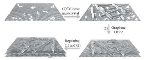
**Figure 4.** Preparation of the laminated cellulose nanocrystals/graphene oxide nanomembranes. Reproduced with permission from [53]. Copyright 2015 John Wiley and Sons.
