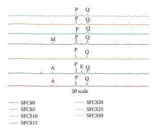
FIGURE 9: XRD analysis result in  $2\theta$  scale. P: portlandite; Q: quartz; A: aluminosilicate; E: ettrignite; M: mullite.
