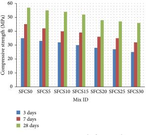
FIGURE 1: Compressive strength of mortar cubes.
