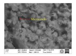
FIGURE 8: SEM image for SFCS30 specimen.
