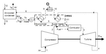
Fig. 1 Layout of Solar STIG cycle [11]
