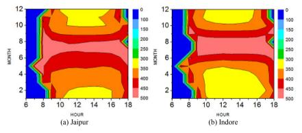
Figure. 7. Annual variation of specific CO<sub>2</sub> emission in kg/MWh, constant power scenario, SAR=0.7
