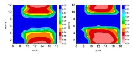
(a) Jaipur (b) Indore Figure. 3. Annual variation of solar to electricity efficiency, constant power scenario, for SAR= 0.7
