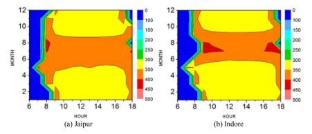
Figure. 8. Annual variation of specific CO<sub>2</sub> emission in kg/MWh, variable power scenario, SAR=0.7
