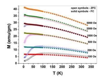
FIG. 4. ZFC-FC curves for RGO-Ni/NF nanocomposite.
