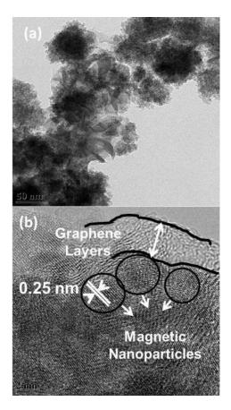
FIG. 2. HRTEM of RGO-Ni/NF nanocomposite at a scale of 50 nm (a) and 2 nm (b).
