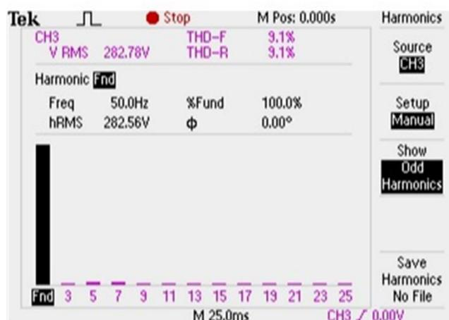
FIGURE 18. Experimental THD of eleven level Inverter
