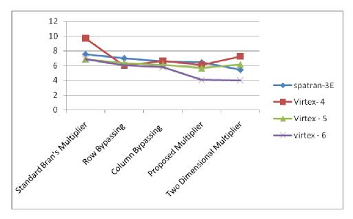
Fig. 12 The average pin delay for Spartan-3AN, Virtex-4, Virtex - 5 and Virtex-6 for standard, row and column bypassing and proposed 4\*4 Braun's multipliers
