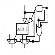
Fig.7 Row & Column Bypassing Adder Cell.
