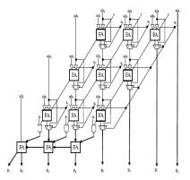
Fig. 3 4\*4 column bypassing
