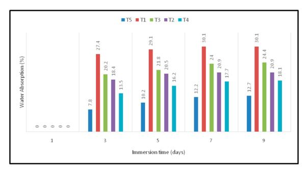
Figure 5. Water absorption (%) of oil palm EFB/kenaf woven fiber-reinforced epoxy-based bi-layer composites.
