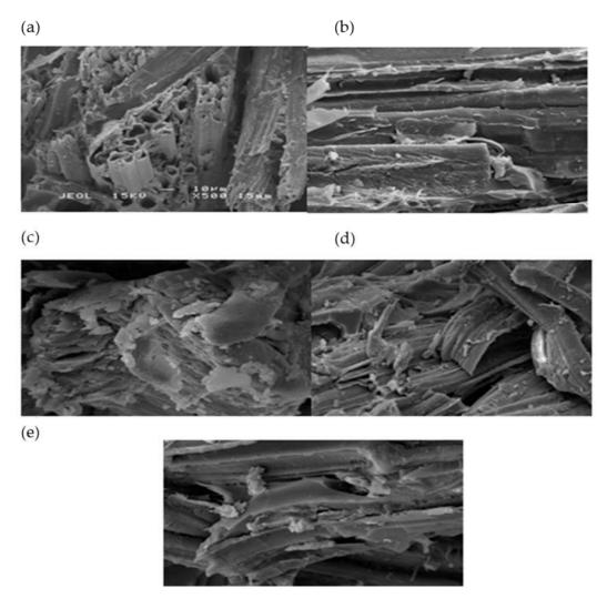
**Figure 2.** Scanning electron micrographs of tensile fracture of T1 composite (**a**), T5 composite (**b**), T2 hybrid composite (**c**), T3hybrid composite (**d**), T4 hybrid composite (**e**), scale bar =  $10 \mu m$ .
