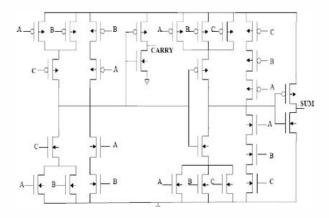
Fig. 1(a) complimentary C-CMOS Full Adder Cell[3].
