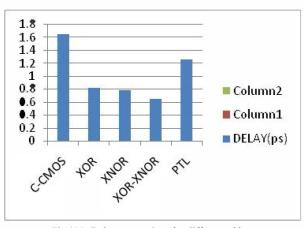
Fig.4(a): Delay comparison for different adders
