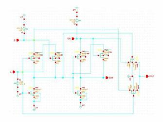
Fig.2(b) EXOR based Full Adder cell
