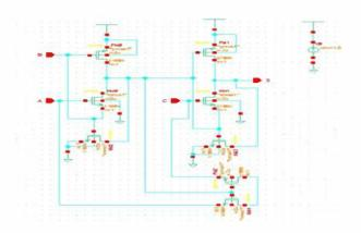
Fig.2(d) EXNOR based Full Adder cell
