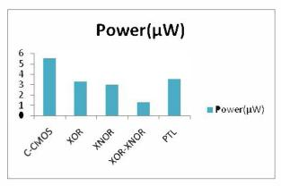
Fig 4(b): Power Comparison results for different adders
