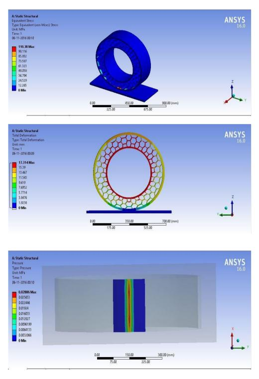
**Figure 4.** Ansys test results for Type B at maximum load showing Von-Mises Equivalent stress, Deformation, and Contact pressure in order.
