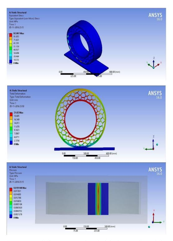
**Figure 3.** Ansys test results for Type A at maximum load showing Von-Mises Equivalent stress, Deformation, and Contact pressure in order.
