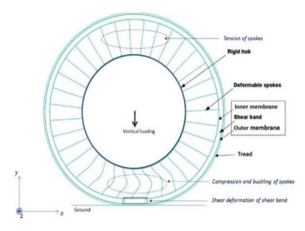
Figure 1. Schematic representation of a non-pneumatic tyre.
