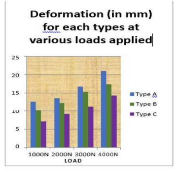
Figure 7. Deformation variation in mm for each type
