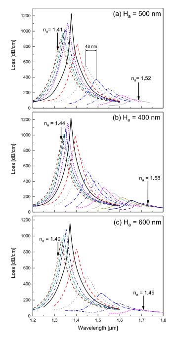
Fig. 5. The loss spectra for the analyte refractive index  $(n_a)$  varying from (a) 1.41 to 1.52 in steps of 0.01, (b) 1.44 to 1.58 in steps of 0.01 and (c) 1.40 to 1.49 in steps of 0.01.
