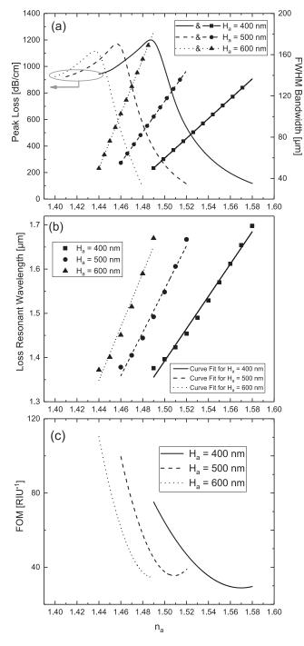
Fig. 6. (a) Peak loss and FWHM Bandwidth for various analyte's RI. (b) Loss resonant wavelengths and straight lines fit. (c) FOM versus analyte's RI for liquid heights  $H_a = 400 \text{ nm}$ , 500 nm and 600 nm, respectively.
