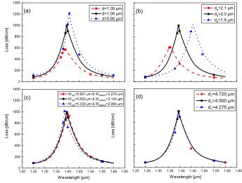
Fig. 9. The investigation on fabrication tolerance of (a) air holes diameter, (b) analyte channel depth, (c) top and bottom base length of trapezoid channel, and (d) side polishing depth.
