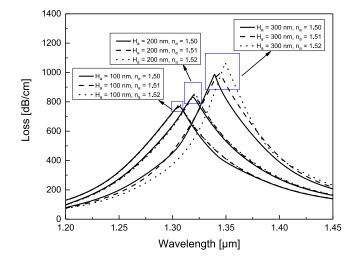
Fig. 7. The loss spectra for the analyte RI varying from 1.50 to 1.52 with different analyte heights of 100 nm, 200 nm and 300 nm.
