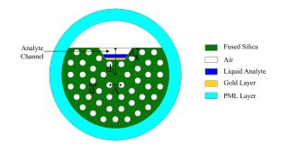
Fig. 1. Cross-section of the proposed six-fold PQF-SPR biosensor.
