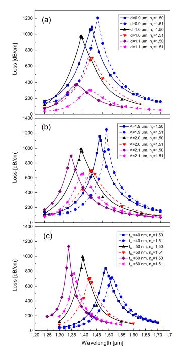
Fig. 8. The loss spectra for (a) three different air holes diameters, 0.9  $\mu$ m, 1.0  $\mu$ m, 1.1  $\mu$ m, (b) three different pitch distances between two adjacent air holes, 1.9  $\mu$ m, 2.0  $\mu$ m, 2.1  $\mu$ m, and (c) three different thin gold coating thickness values, 40 nm, 50 nm, 60 nm with a liquid analyte height of 400 nm and RI of 1.50 and 1.51.
