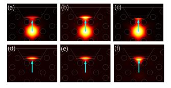
Fig. 3. Light energy flow distributions in the cross-section of PQF-SPR biosensor for different wavelengths for the analyte RI of  $n_a = 1.49$  and height 500 nm. (a) and (d) are the FM and PM at 1370 nm (shorter wavelength with respect to the resonance). (b) and (e) are the FM and PM at resonant wavelength of 1492 nm. (c) and (f) are the FM and PM at 1650 nm (longer wavelength with respect to the resonance).
