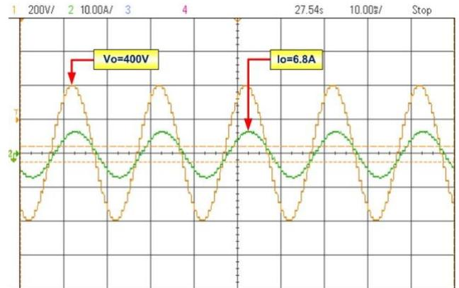
**FIGURE 18.** Experimental output waveform with L Load
