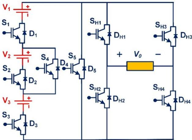
FIGURE 6. The basic structure of 5-level MLI
