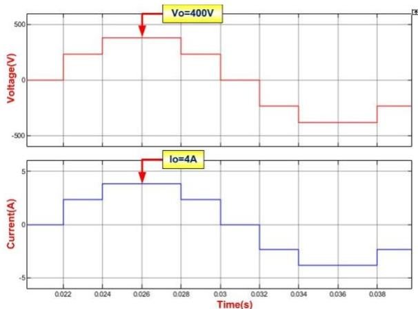
FIGURE 8(a). Simulation output voltage and current waveforms of a five-level inverter
