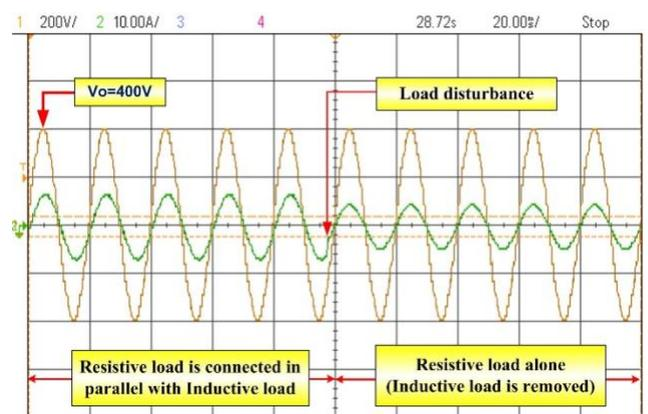
**FIGURE 20.** Experimental output waveform with L||R Load
