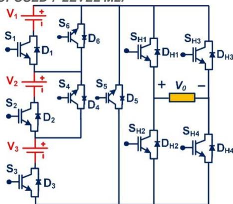
FIGURE 9. The basic structure of 7-level MLI
