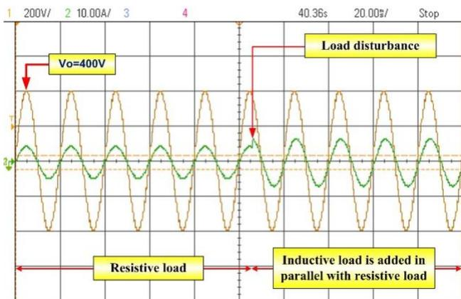
**FIGURE 19.** Experimental output waveform with R||L Load
