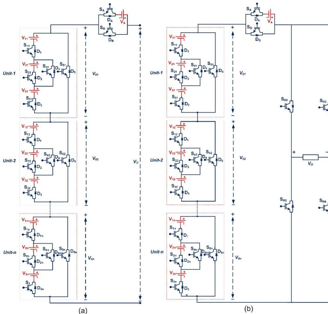
FIGURE 5.1. Developed Cascaded Multilevel Inverter.
