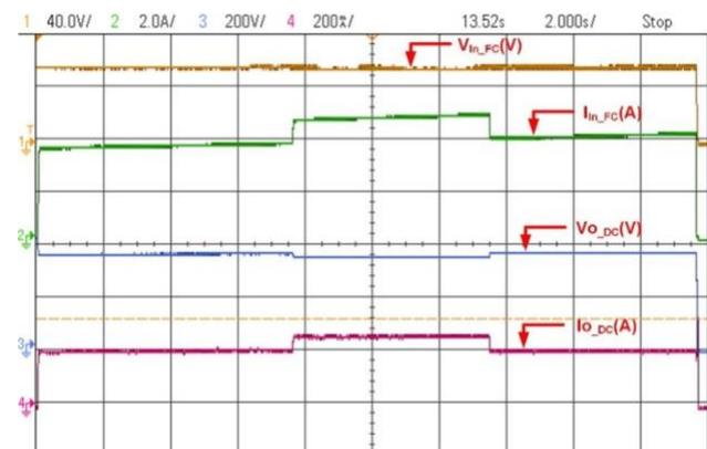
FIGURE 4. The 4-level converter & FC Simulation waveforms
