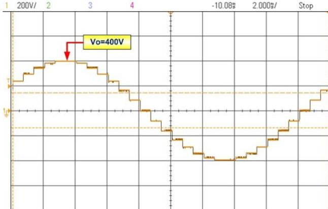
**FIGURE 16.** Experimental output waveform ( $V_o$ )
