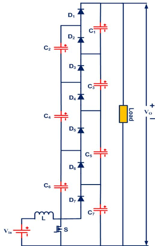
FIGURE 2. 4-level Boost Converter [33]
