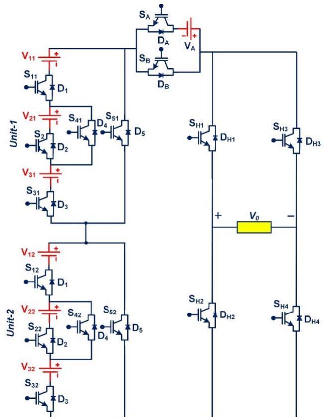
FIGURE 12. The basic structure of 15-level MLI
