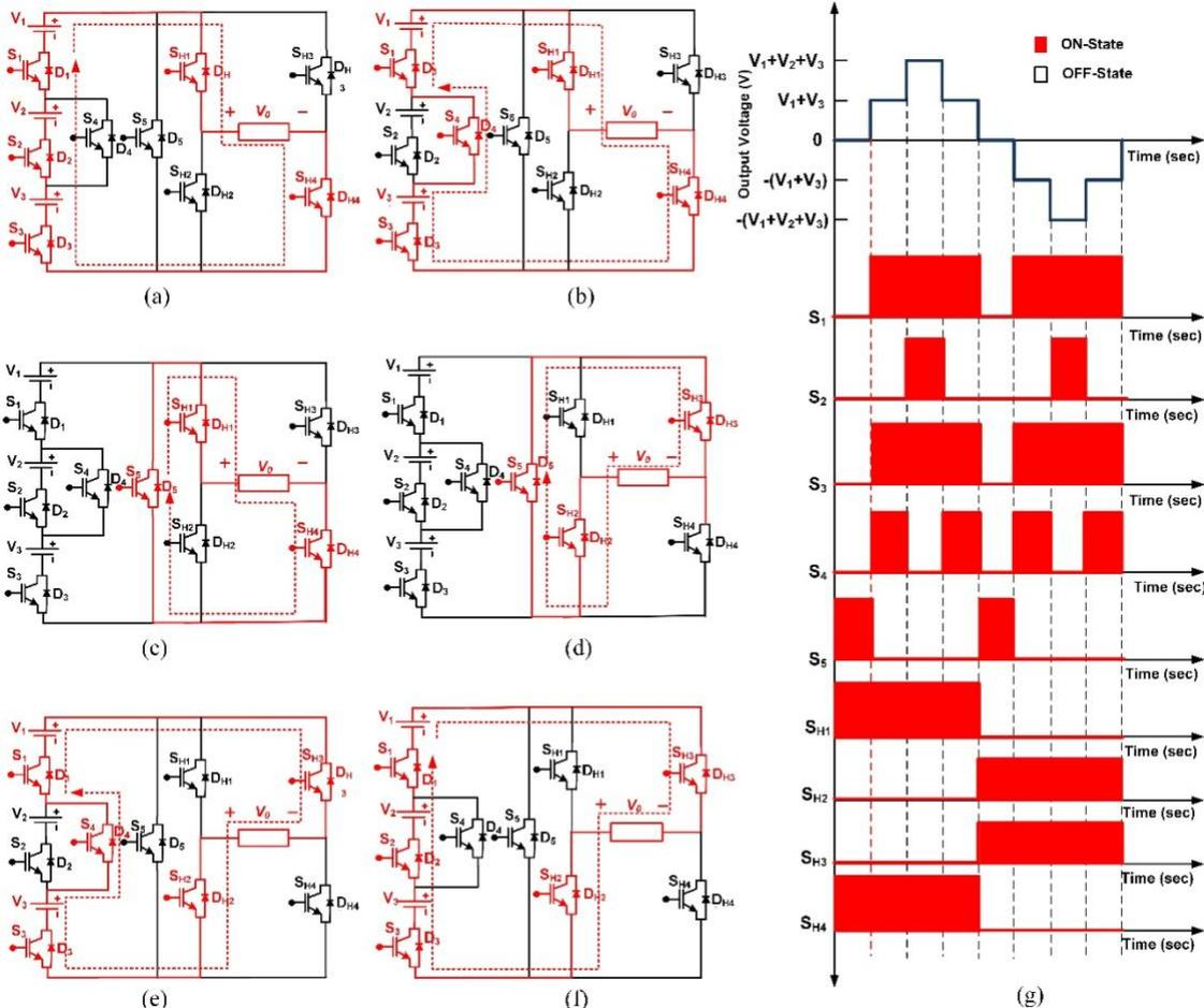
FIGURE 7. Modes of operation of the developed 5-Level MLI topology (a): Mode-1, (b) Mode-2, (c) Mode-3, (d) Mode-4, (e) Mode-5, (f) Mode-6, (g) 5-Level expected output voltage waveform
