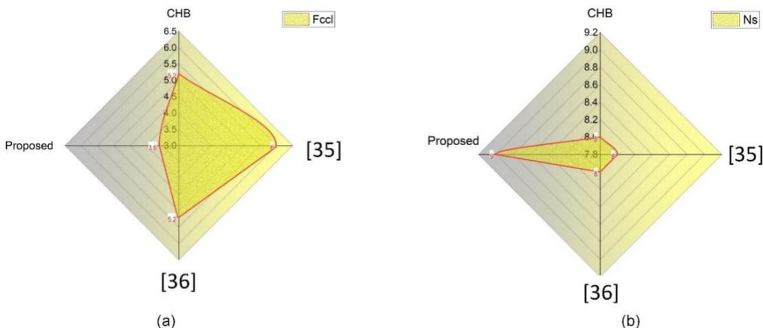
FIGURE 23. (a) Comparison of components count per level of proposed MLI with other topologies. (b) Comparison of Number of Switches to the proposed MLI with other topologies.
