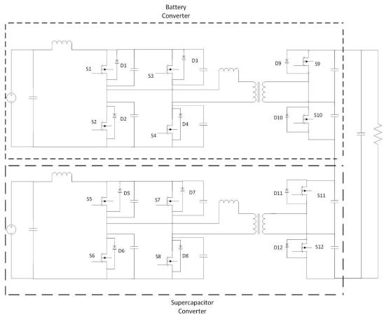
Figure 8. Bidirectional ESS converter
