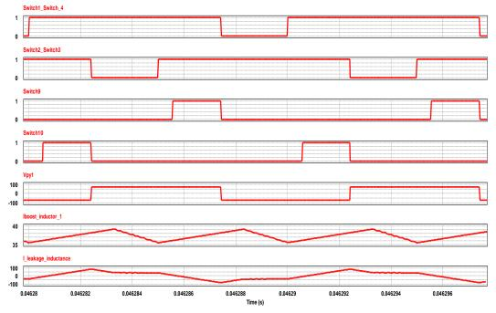
Figure 17. Switching pattern, Primary voltage, boost inductor current and leakage inductor current of super capacitor converter
