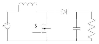
Figure 3. Unidirectional FC converter
