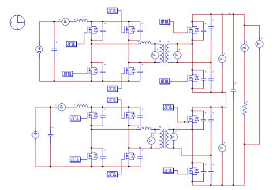
Figure 15. Circuit model of bidirectional converter developed in PSIM
