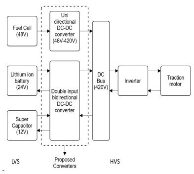
Figure 2. Powertrain structure of a fuel cell hybrid electric vehicle
