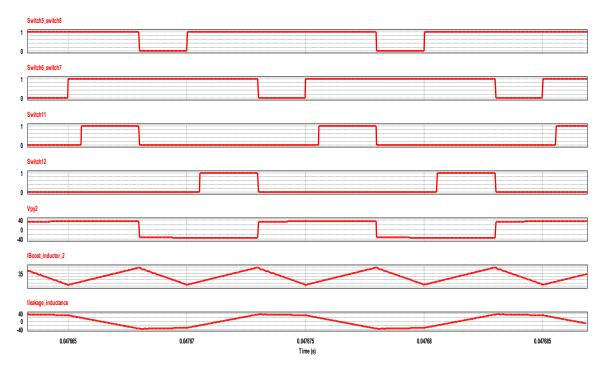
Figure 16. Switching pattern, Primary voltage, boost inductor current and leakage inductor current of super capacitor converter
