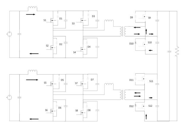
Figure 9. Mode 1 circuit diagram
