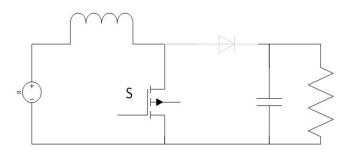
Figure 4. Mode1-Switch is turned on
