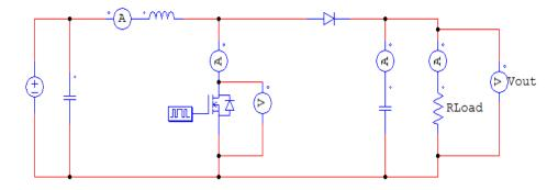
Figure 6: Simulation circuit model of unidirectional FC converter developed in PSIM
