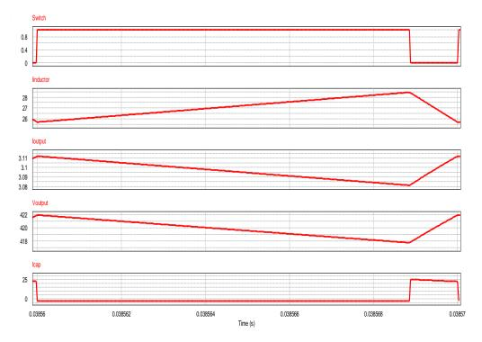
Figure 7. Switching pulse pattern, Inductor current, output current, output voltage and capacitor current of the unidirectional FC converter
