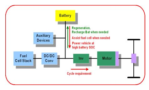
Figure 2. Fuel cell power conversion system components.
