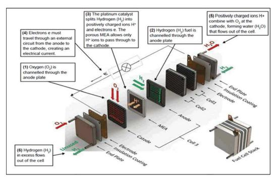
Figure 1. Layout and operation of PEMFC.
