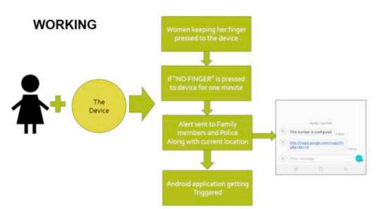
Fig. 4. Workflow of the Proposed Design
