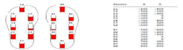
Figure 5: Vertical Ground Reaction Force for 8 sensor location under each foot[17] Figure 6 : Locations of 8 load sensors on each foot where "L" and "R" denotes left and right respectively[11].
