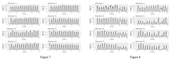
Figure 7 (Left Side): Vertical Ground Reaction Force (VGRF) in Newton of first 2000 instance of time in seconds with 8 sensors placed under right foot of healthy subject.
