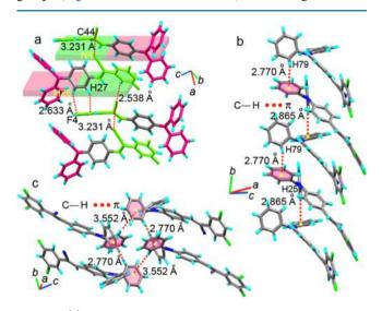
**Figure 3.** (a) Intermolecular interactions in the crystal structure of 10. Arrangement of donor-acceptor groups are colored red and green, respectively. (b, c) C-H $\cdots\pi$  interactions along different crystallographic directions.
