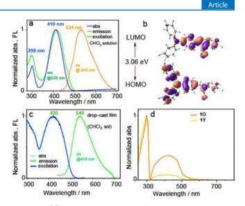
Figure 1. (a) Solution-state UV–vis, fluorescence, and excitation spectra of 1 (CHCl<sub>3</sub>  $1 \times 10^{-5}$  M solution); (b) DFT-calculated HOMO and LUMO orbitals of 1; (c) UV–vis, fluorescence, and excitation spectra of 1 drop-cast thin film (from CHCl<sub>3</sub>  $1 \times 10^{-3}$  M solution); and (d) solid-state absorption spectra of small crystals of 1Y and 1O.
