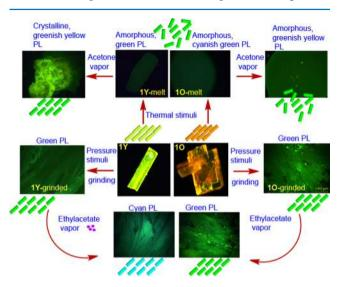
Figure 7. Multistimuli (pressure-, vapo-, thermo-) responsive behavior and possible changes in the molecular arrangement in 1O and 1Y crystal/powder.
