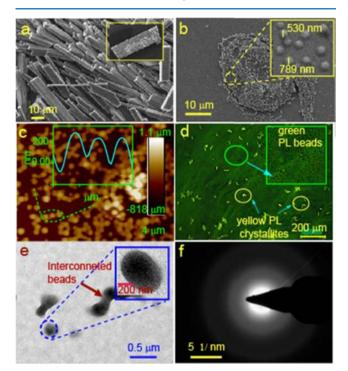
Figure 6. (a) SEM image of crystallites of 1 obtained by drop casting from DMF solution. (b, c) SEM and atomic force microscopy (AFM) images of bead-shaped particles of 1 from methanol solution. (d) Fluorescence microscopy image of drop-cast (from methanol) solid; amorphous beads show green fluorescence and crystallites show yellow fluorescence. (e) TEM image of beads and (f) selected area electron diffraction (SAED) image of the bead particles.
