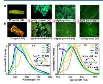
Figure 2. Fluorescence microscopy images and corresponding spectra of multistage mechanochromic luminescence. (a) **1Y** crystal and (b) **1O** crystal. The stepwise color changes are given in subpanels (a1-a4) and (b1-b4). (c) Fluorescence spectra for **1Y** in different stages of grinding with reference to (a1-a4). (d) Fluorescence spectra for **1O** crystals with reference to (b1-b4).
