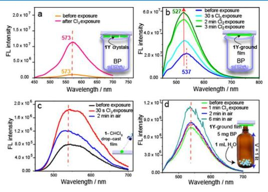
**Figure 8.** Chlorine gas (evolved from bleaching powder and water) sensing by 1. (a) PL spectral change of **1Y** crystal before and after exposure. Bleaching powder is abbreviated as BP in the figure panels. (b, c) Same for **1Y**-ground film and **1** drop-cast film (from chloroform solution). (d) **1Y**-ground film with approximately 1.7 ppm (in air) chlorine concentration.
