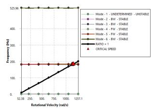
Figure 4. Campbell diagram of conventional steel shaft
