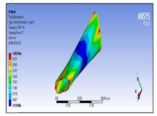
Figure 16. Fifth mode shape- FG shaft
