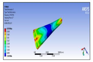
Figure 8. Third mode shape - conventional steel shaft
