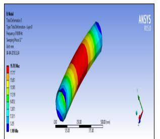
Figure 13. Second mode shape- FG shaft
