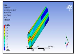
Figure 15. Fourth mode shape-FG shaft
