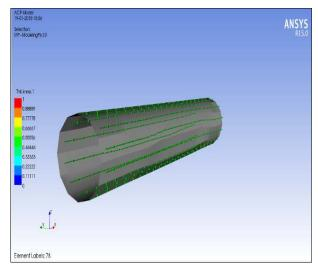
Figure 2. Fibre direction is along reference axis (X axis)
