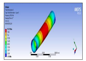
Figure 14. Third mode shape- FG shaft
