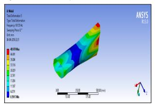
Figure 10. Fifth mode shape- conventional steel shaft
