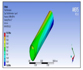
Figure 12. First mode shape- FG shaft
