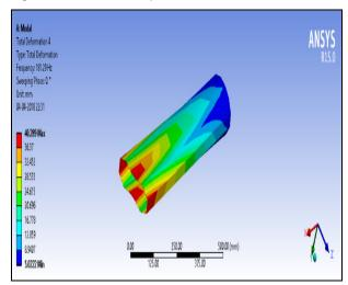
Figure 9. Fourth mode shape- conventional steel shaft
