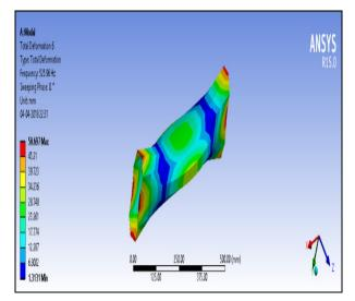
Figure 11. Sixth mode shape- conventional steel shaft
