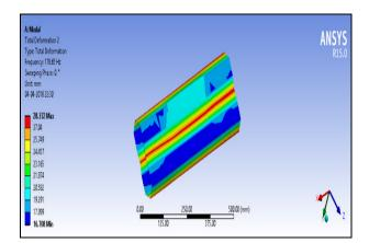
Figure 7. Second mode shape - conventional steel shaft
