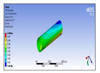
Figure 6. First mode shape - conventional steel shaft
