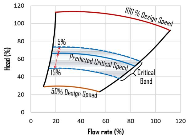
**Figure 5.** Critical speed band curve
