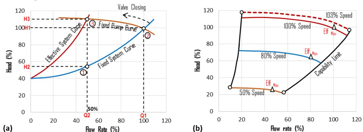
**Figure 2.** Centrifugal pump operation (a) variable speed and (b) fixed speed
