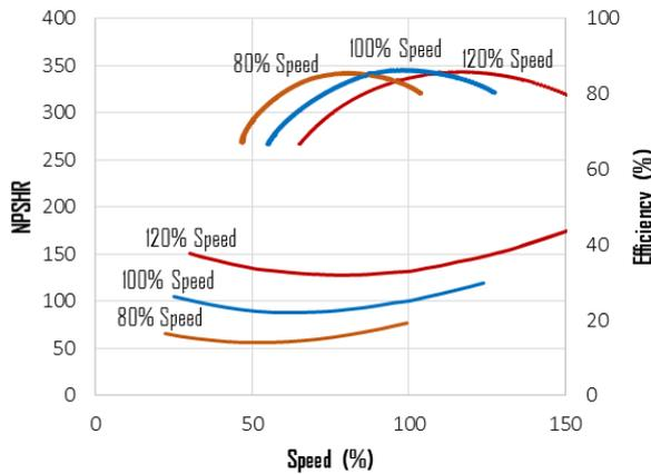
**Figure 3.** NPSHR – Efficiency Vs Speed
