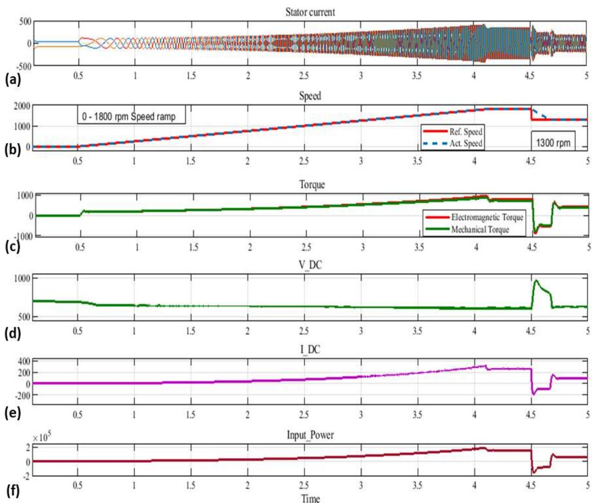
**Figure 8:** Simulated results of sensorless pump drive
