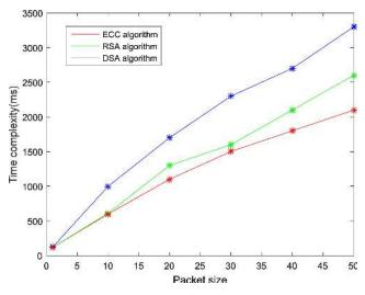
FIGURE 6. Time Complexity of ECC compared to RSA and DSA, as evaluated in [42].
