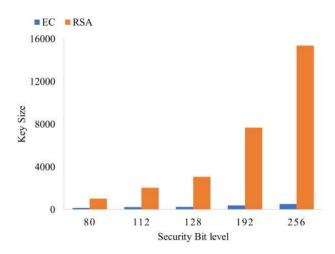
FIGURE 7. Comparison of RSA and EC.
