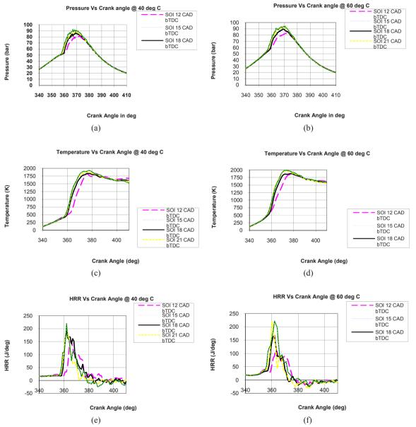
Fig.2 (a) In-cylinder pressure at  $40^{\circ}$ C of air intake temperature, (b) In-cylinder pressure at  $60^{\circ}$ C of air intake temperature, (c) Combustion temperature at  $40^{\circ}$ C of air intake temperature, (d) Combustion temperature at  $60^{\circ}$ C of air intake temperature, (e) HRR at  $40^{\circ}$ C of air intake temperature, (f) HRR at  $60^{\circ}$ C of air intake temperature.
