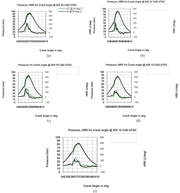
Fig.3 (a), (b), (c), (d), (e) In-cylinder pressure and heat release rate at different SOI and AIT
