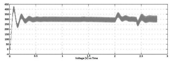
Fig 4. Output voltage of Boost converter
