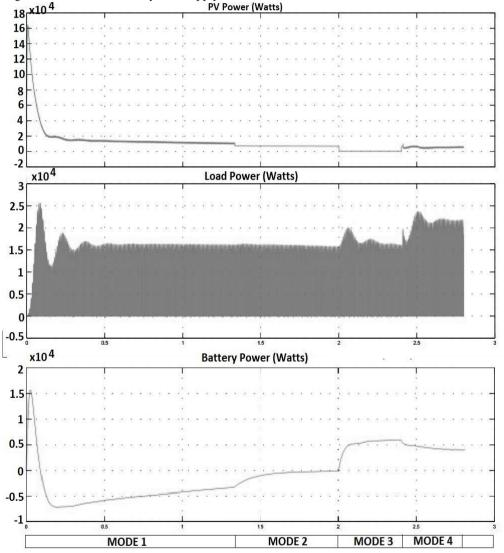
Fig 7. Output power vs simulation time graph of PV, load and battery during the entire simulation.
