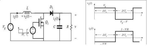
Fig 3. (a) Circuit diagram of a (DC-DC) Boost Converter; (b) V-I graph.
