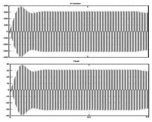
Fig 5. Output voltage and current of load in Mode 1
