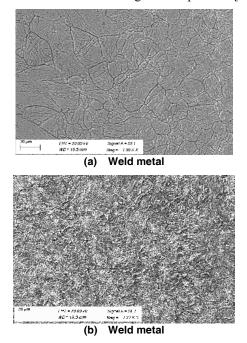
Figure 8: SEM image Helium weld Specimen
