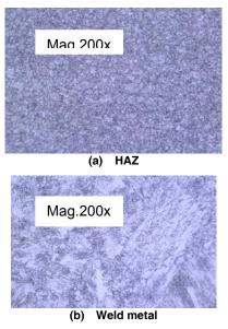
Figure 6: Microstructure image of Argon 50% & Helium 50% gas specimen HAZ and WM
