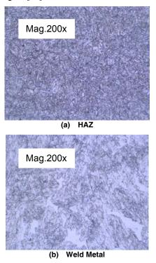
Figure 5: Microstructure of Helium gas specimen HAZ &WM
