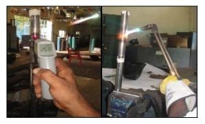
Figure 1: Pre heating the test specimen
