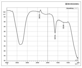
Fig. 2: Fourier Transform infrared spectrum of *Ipomoea nil* aqueous extract
