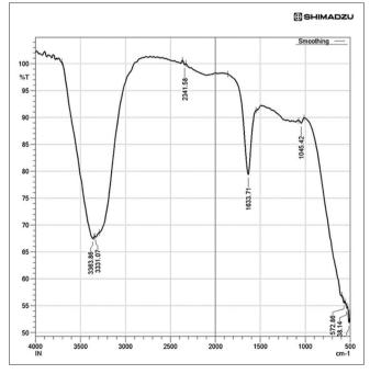
Fig. 3: Fourier Transform infrared spectrum of silver nanoparticle
