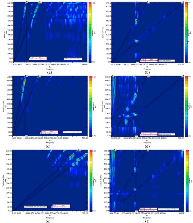
**Figure3.** Campbell diagram illustrating orders of frequency at different locations. Campbell diagram at hub for, (a) conventional scooter (b) electric scooter. Campbell diagram at seat for, (c) conventional scooter (d) electric scooter. Campbell diagram at handlebar for, (e) conventional scooter (f) electric scooter.
