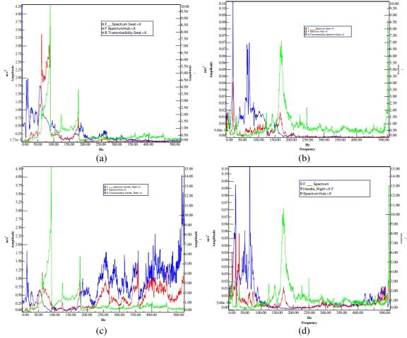
**Figure 4.** Acceleration responses on the left vertical axis and transmissibility ratio of target locations on the right vertical axis. Transmissibility at the seat for (a) conventional scooter, (b) electric scooter. Transmissibility at handlebar for (c) conventional scooter, (d) electric scooter.
