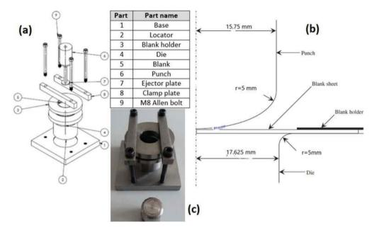
**Figure 1.** (a) Exploded view of forming tool with blank holding system (b) Geometry of forming tools (c) Assembled forming tools.
