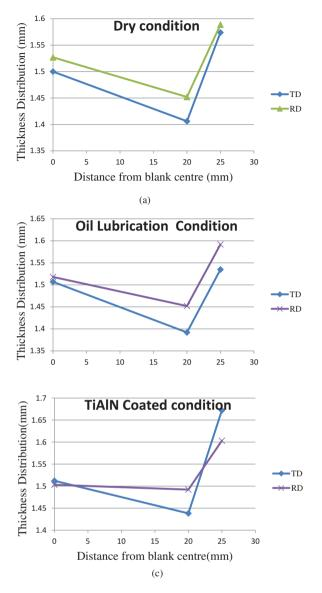
**Figure 4.** (a) Thickness variation under dry condition. (b) Thickness variation in oil-lubricated condition. (c) Thickness variation with TiAIN-coated condition.
