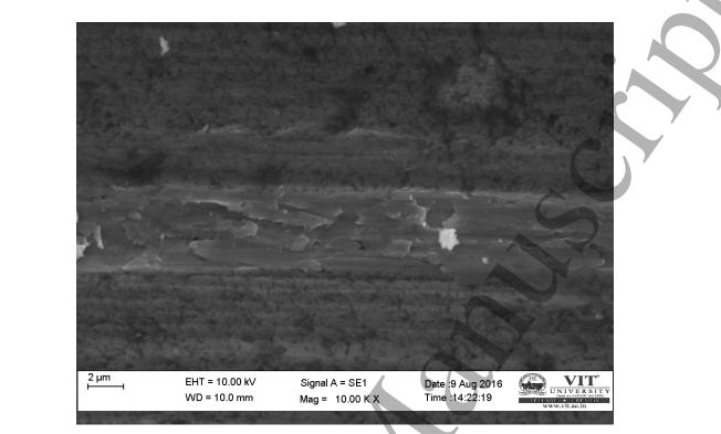
Figure 18: SEM Micrograph of the AA LM6 P/M Pin wear track
