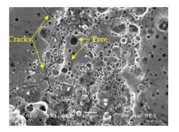
Fig. 11 SEM micrographs showing pores and cracks for experiment number 22
