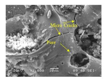
Fig. 10 SEM micrographs showing pores and cracks for experiment number 22
