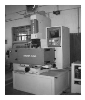
Fig. 1 EDM machine set-up
