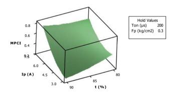
Fig. 8 Surface plot of MPCI vs  $I_{p}$ ,  $\tau$
