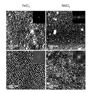
Fig. 1 AFM images demonstrating the poor lateral order of micellar monolayers on Si substrates loaded *directly* into solution with FeCl<sub>3</sub> (a) and NbCl<sub>5</sub> (b) metal precursors ('conventional' technique). Using our new approach, a significantly improved lateral order can be achieved for both FeCl<sub>3</sub> (c) as well as NbCl<sub>5</sub> (d) loaded micelles. The insets represent the auto-covariance functions of the corresponding AFM images.
