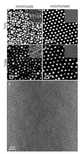
Fig. 2 AFM images and related auto-covariance functions (insets) of micellar patterns obtained from PS(185 000)-*b*-P2VP(90 000) based solutions that are loaded by FeCl<sub>3</sub> and NbCl<sub>5</sub>, using hP2VP(1200) (a and b) and hP2VP(97 000) (c and d) as precursor carriers; (e) represents a larger scan range of the sample shown in (c).
