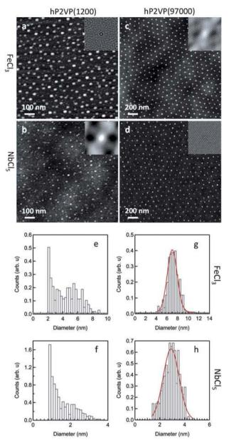
Fig. 3 AFM images (a–d) and size distributions (e–h) of iron oxide (a, c, e and g) as well as niobium oxide (b, d, f and h) nanoparticles obtained after oxygen plasma treatment of micellar monolayers prepared using hP2VP(1200) (left row) and hP2VP(97 000) (right row) as carriers for the metal salts. Assuming Gaussian profiles, average particle diameters of 7.0  $\pm$  0.66 nm (g) and 3.0  $\pm$  0.45 nm (h) can be derived for the different material systems.
