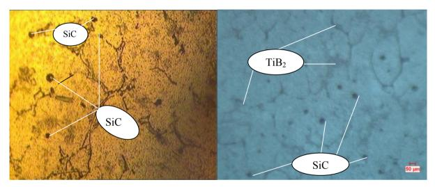
Fig.1(a) Optical micrograph of 10SiC-0TiB<sub>2</sub>
