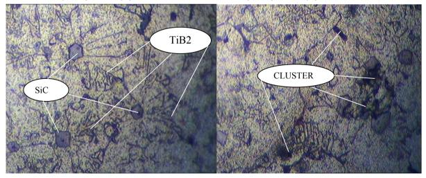
Fig. 1(c) Optical micrograph of (10SiC-5TiB<sub>2</sub>).
