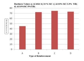
Fig. 2 Shows the micro hardness plot of specimens
