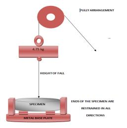
**Figure 2.** Schematic representation of impact toughness set up.
