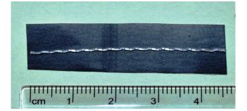
Figure 1. Crimped polypropylene fibre.
