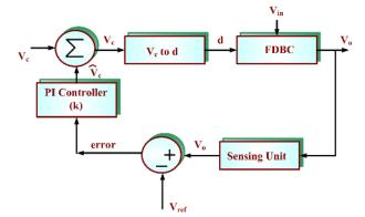
FIGURE 4. Closed loop system of FDBC.
