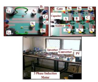
FIGURE 8. Experimental setup of proposed work.
