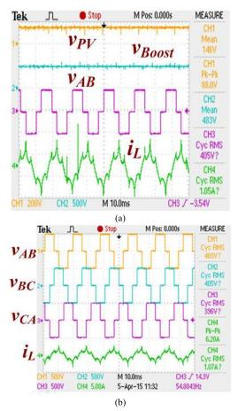
FIGURE 11. Output waveform of the entire system (a) output waveform of the PV voltage, FDBC voltage, VSI voltage and current, (b) motor output waveform.
