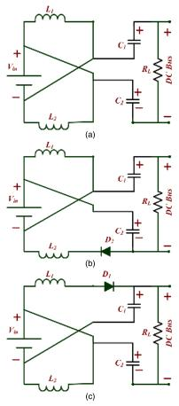
FIGURE 3. FDBC equivalent circuit (a) mode 1, (b) mode (2), (c) mode 3.
