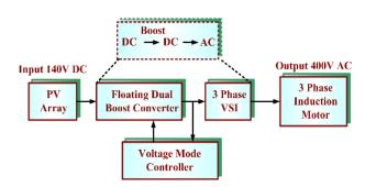
FIGURE 1. Block diagram of PV integrated controlled converter system.
