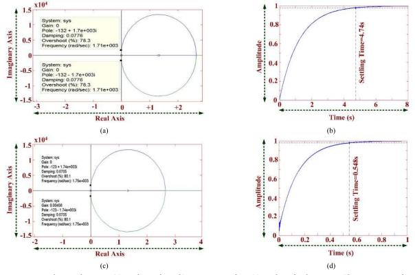
FIGURE 7. Root locus and response (a) root locus of  $TF_c$ , (b) step response of  $TF_c$ , (c) root locus for the new  $TF_c$ , (d) step response of the new  $TF_c$ .
