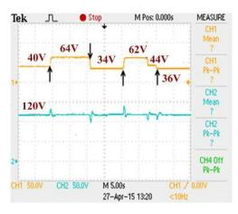
FIGURE 12. Closed-loop output waveform of FDBC in hardware.
