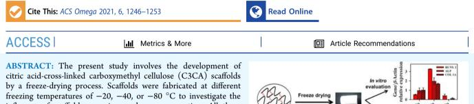
influence of scaffold pore size on bone regeneration. All three scaffolds were porous in structure, and the pore size was measured to be 74  $\pm$  4, 55  $\pm$  6, and 46  $\pm$  5  $\mu$ m for -20, -40, and -80 °C scaffolds. The pores were larger in scaffolds processed at -20 °C compared to -40 and -80 °C, indicating the reduction in pore size of the scaffolds with a decrease in freezing temperature. The
