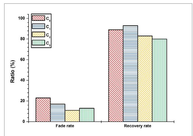
Fig. 7. Friction parameters of BFM composites.
