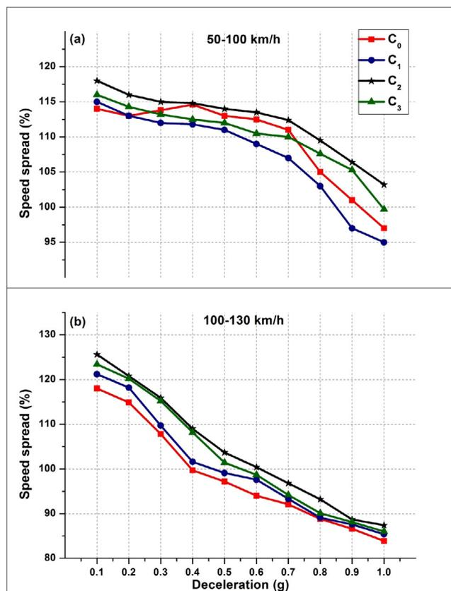
**Fig. 4.** Speed sensitivity of the friction composites at (a) mild condition (b) severe condition.
