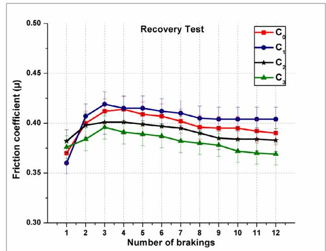
Fig. 6. Recovery of the developed BFM composites.
