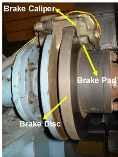
Fig. 2. Rotor disc and pad arrangement in dynamometer.
