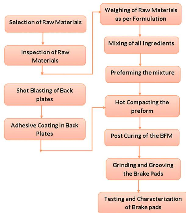
**Fig. 1.** Manufacturing process flowchart.
