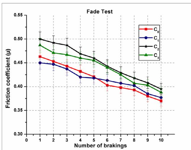
Fig. 5. Fade of the developed BFM composites.
