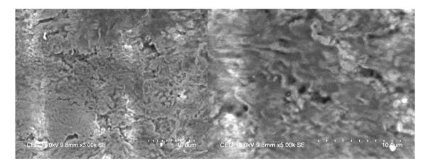
Fig. 6 SEM Image at the middle of the wear track 3000X and 5000X
