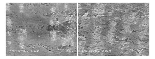
Fig. 7 SEM image at the right and left end of the wear track
