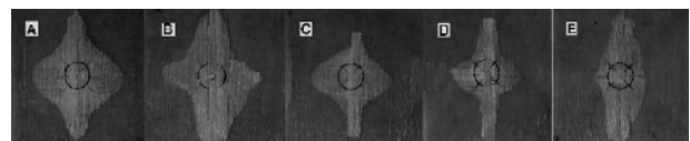
Fig. 7: Back face damage of (A) truncated conical, (B) truncated ogival, (C) hemispherical, (D) conical, (E) ogival for plates of 5.35 mm plates.
