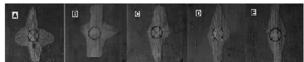
Fig. 8: Back face damage of (A) truncated conical, (B) truncated ogival, (C) hemispherical, (D) conical, (E) ogival for plates of 3.64 mm plates.
