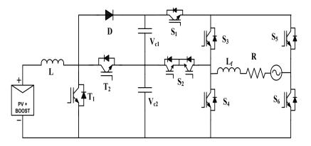
Fig. 4 Proposed multilevel inverter with dual boost converter
