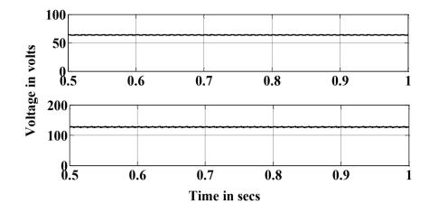
Fig. 6. Dual output boost converter output voltage waveform (upper and bottom: Vc1 & Vc2)
