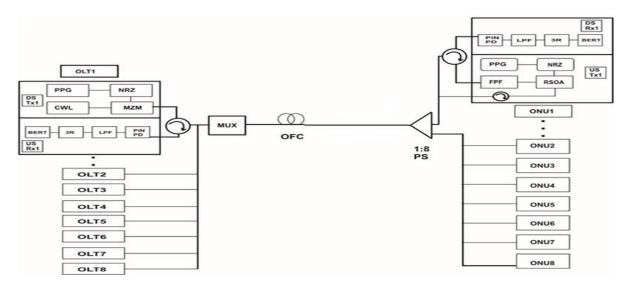
Fig. 1. The Schematic Stacked Wavelength Model for NG-PON2.
