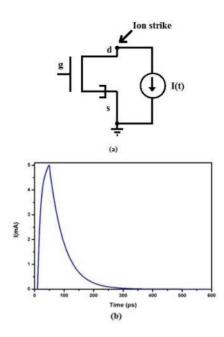
FIGURE 9. (a) Ion strike tunneling by a current source (b) current pulse.
