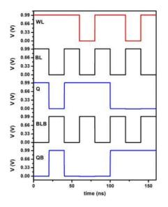
FIGURE 8. Timing diagram of 6T TFET SRAM.
