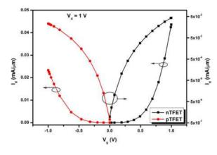
FIGURE 4. Id-Vg characteristics of n- and p-type DG TFETs.
