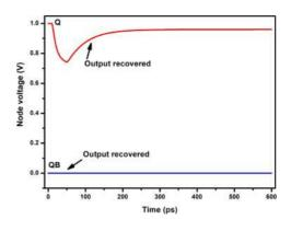
FIGURE 13. Node voltages of radiation hardened 6T TFET SRAM cell.
