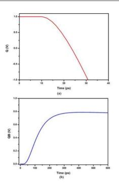
FIGURE 11. Node voltages due to SEU (a) '1' to '0' upset at Q (b) '0' to '1' upset at QB.
