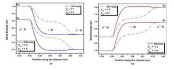
FIGURE 3. Simulated energy band diagram (a) n-type DG TFET (b) p-type DG TFET.
