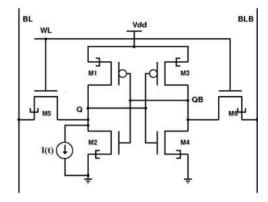
FIGURE 10. 6T TFET SRAM cell with injected current source.
