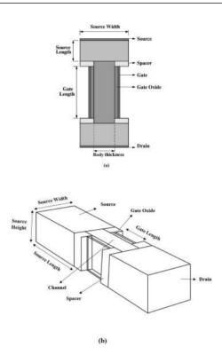
FIGURE 2. Schematic structure of DG TFET (a) 2D view (b) 3D view.
