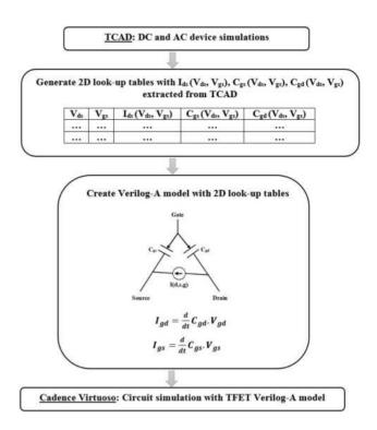
FIGURE 5. Flowchart for look-up table based Verilog-A model generation from TCAD simulations.
