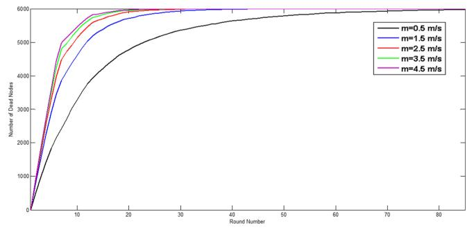
Fig. 12. Number of dead nodes for different values of mobility for IMCP algorithm.
