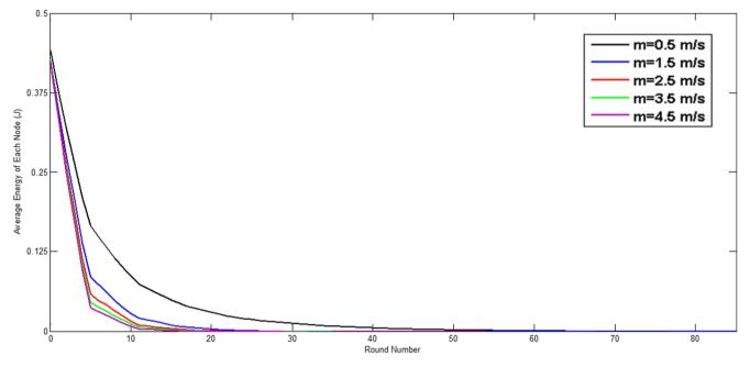
Fig. 13. Average energy of nodes for IMCP with varying mobility speeds.
