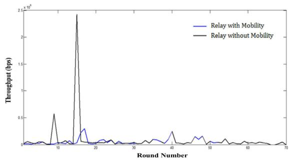
Fig. 17. Throughput (bps) for IMCP process for three tier system considering with and without mobility parameter.
