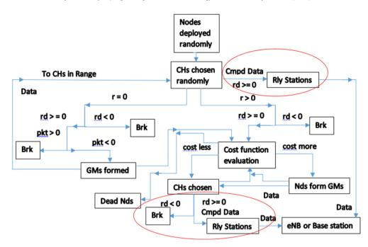
Fig. 6. Chart of the proposed clustering process involved in M2M communication for three tier systems.
