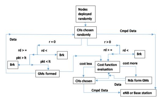
Fig. 4. Chart of the proposed clustering process involved in M2M communication.
