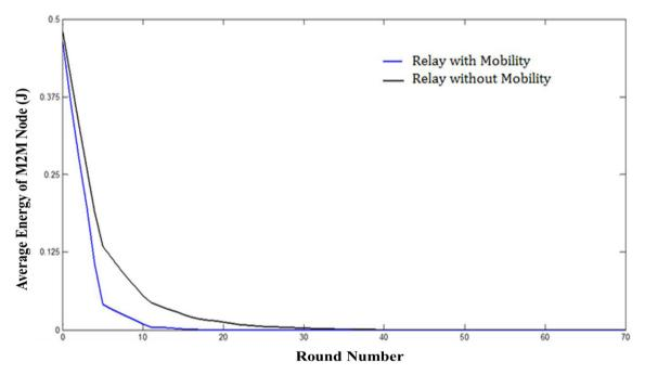
Fig. 16. Average energy of nodes for IMCP process for three tier system (with relay (rly)).
