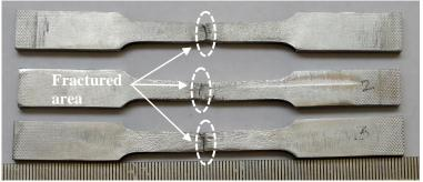
Figure 5 Photograph of failure tensile tested specimens of ATIG welded C-276 alloy
