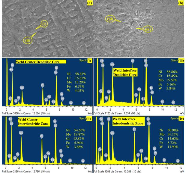
Figure 4 SEM/EDAX analysis of ATIG welded C-276 alloy for different places of weldment a) SEM-Weld Center; b) SEM-Weld Interface; i)Weld Center- Dendritic Core; ii) Weld Center- Interdendritic Zone; iii)Weld Interface- Dendritic Core; iv) Weld Interface- Interdendritic Zone
