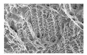
Figure 6 SEM fractograph of tensile tested specimen
