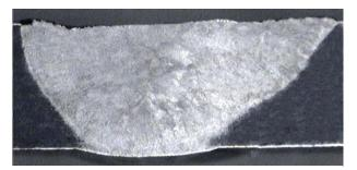
Figure 2 Macrostructure of the ATIG welded alloy C-276
