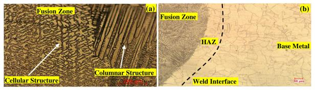
Figure 3 Microstructure of ATIG welded alloy C-276 alloy a) Fusion Zone; b) Weld Interface
