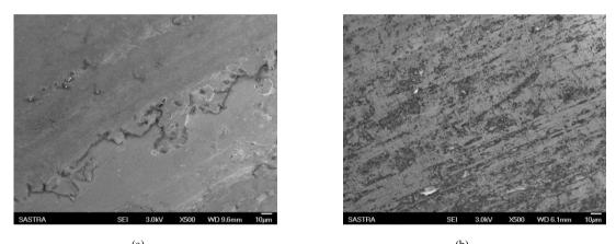
(a) (b) Figure- 6 SEM images of extruded P/M alloy steels wear track: (a) Fe-1%C-1%W; (b) Fe-1%C-1%Ti
