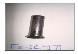
(a) (b) Figure- 1 Extruded P/M alloy steels (a) Fe-1%C-1%W; (b) Fe-1%C-1%Ti
