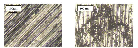
(a) (b) Figure- 5 Wear pattern of maximum worn out of extruded P/M alloy steels (a) Fe-1%C-1%W; (b) Fe-1%C-1%Ti
