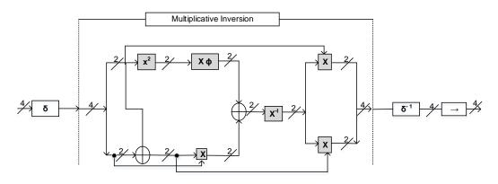
**Figure 2.** Proposed S-box structure in finite fields. The affine and the inverse transformations are carried out in the field GF ( $2^4$ ) and the multiplicative inversion is carried out in the composite field GF ( $(2^2)^2$ ).
