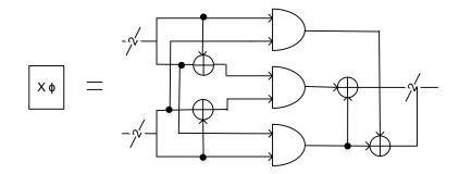
**Figure 4.** Multiplier in the composite field GF  $((2^2)^2)$ . The 2 × 2 multiplier in the GF  $((2^2)^2)$  employs three XOR gates and three AND gates.
