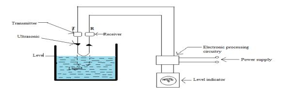
Figure 11: Ultrasonic type level measurement.
