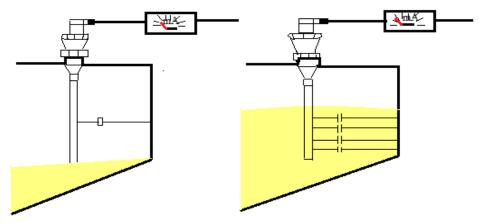
Figure 4: Electrical capacitance method.
