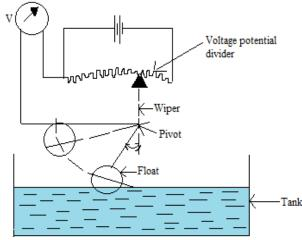
Figure 12: Float actuated resistive level measurement.
