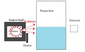
Figure 5: Radiation level measurement.
