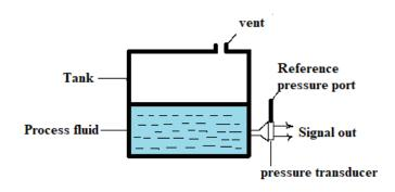
Figure 3: Level measurement using pressure transmitter.
