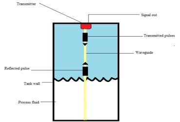
Figure 13: Radar type of level measurement.
