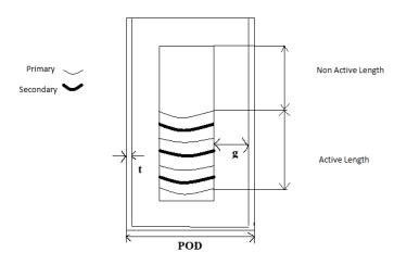
Figure 14: Schematic of Mutual inductance level probe (MILP).
