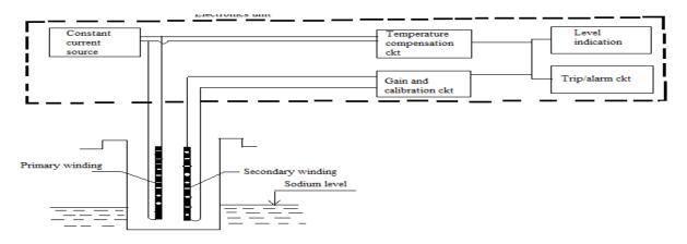
Figure 15: Mutual inductance type continuous level probe.
