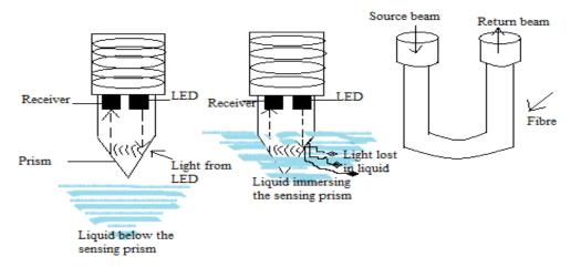
Figure 10: Optical type level measurement.
