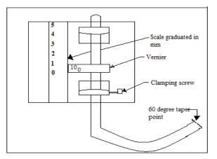
Figure 2: Hook-type level measurement.
