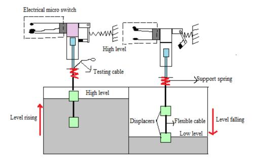
Figure 8: Float displacement type level measurement.
