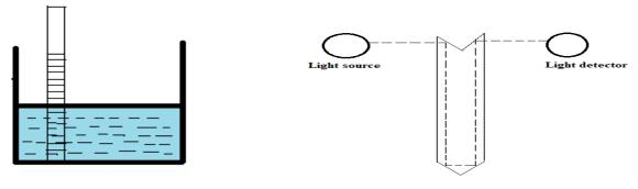
Figure 6: Dipstick level measurement.
