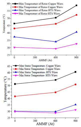
Figure 5. Temperature distribution on Rotor core and Stator core with HTS Copper wires [19]
