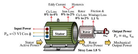
Figure 6. Typical loss component of 37.5 kW three phase squirrel cage induction motor
