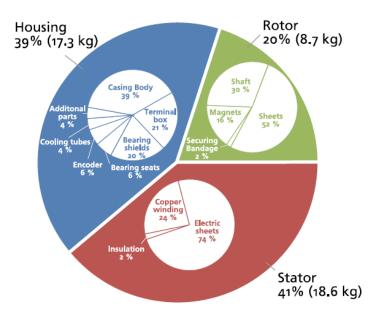
Figure 1. Distribution of weight of an electric motor [2]
