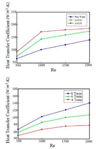
Figure 3. Effect of heat transfer with and without Aluminum-Oxide nano-particles [15]
